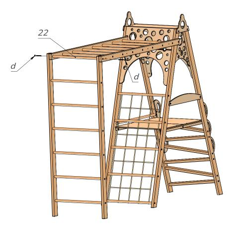
Attach the semi-product shown in the Pic.17 to the previously assembled construction. Before that, install the nog (22) with the screw (d) and hex key (g). See Pic.19.
