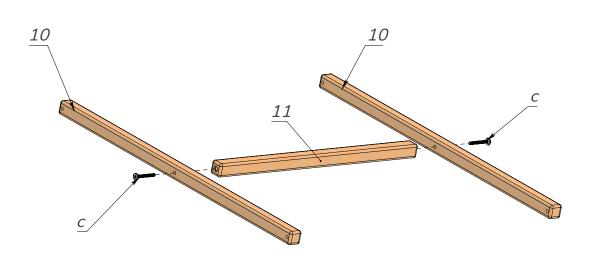
Take the lintel (11) and using the screws (c) and hex key (g) attach the middle planks (10). See Pic.7.
