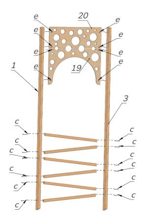
Install the sidewalls #2, #3 (19, 20) between the stands (1, 3) and close the eccentric ties (e) clockwise by turning them by 180 degrees. Then attach the askew planks (12) with the help of screws (c) and hex key (g). See Pic.3.
