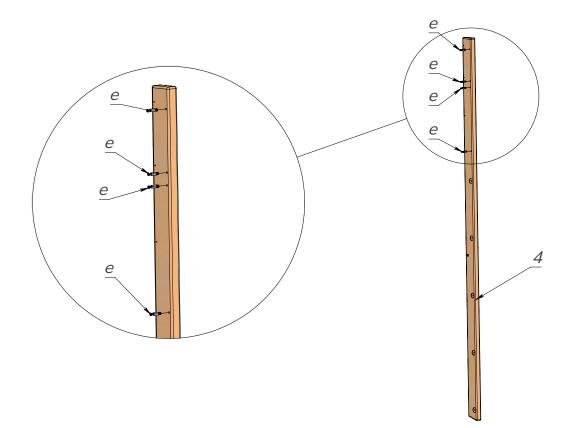
Take the stand (4) and using the screwdriver (h) install the dowels from minifixes (e). See Pic.5.
