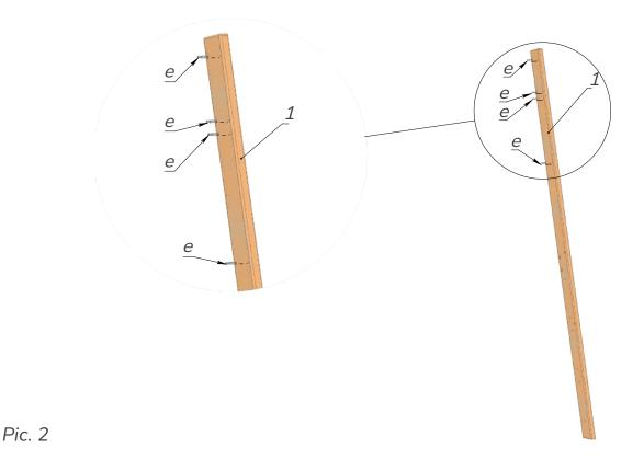
Take the snatd (1) and using the screwdriver (h) install the dowels from minifixes (e). See Pic.2.
