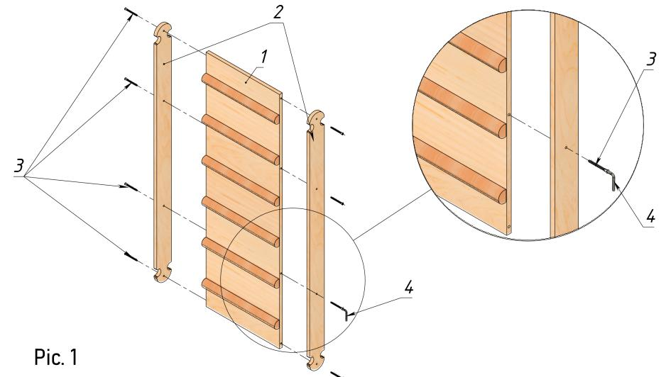
Take one of the Sidewalls (2) and connect it to the Ramp (1) using the Confirmat screws (3) and Hex key (4). Another Sidewall (2) connect with the previously assembled construction with the Confirmat screws (3). See Pic. 1
