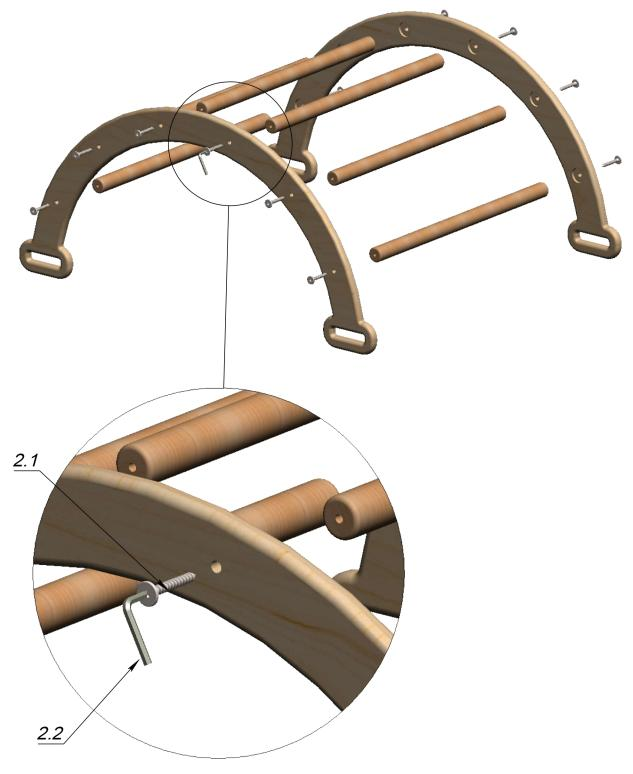
Screw two parts 1.1(p.1) to parts 1.2(p.1) with screws 2.1(p.1) using a Hex key 2.2(p.1)
