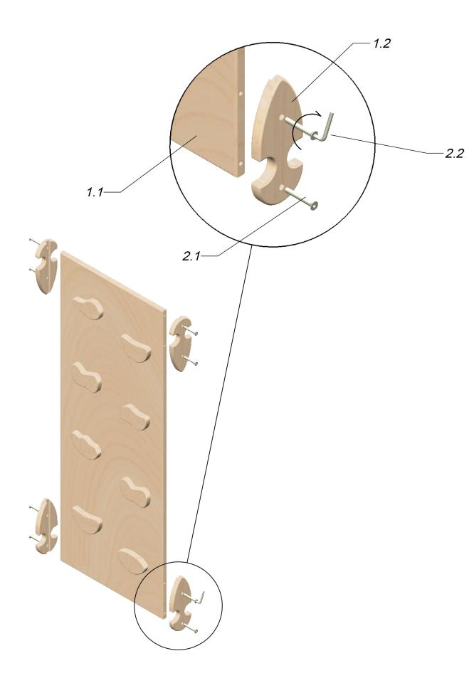
Screw the hooks (1.2) to the Ramp (1.1) with the confirmat Screws (2.1). Tighten with the 3mm hex key (2.2).
