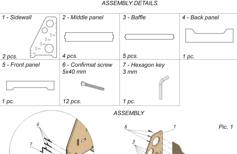
1. Take one of the Sidewalls (1), Middle panel (4) and Front panel (5) using the Confirmat screws (6) and Hexagon key (7).
