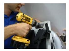
3. Remove the bracket and drill two  $\frac{1}{4}$ " holes in the blower back plate where the marks were made in Step 2.
