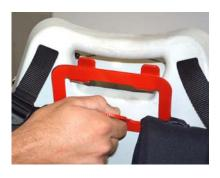
1. Position the bracket so that the fingers hook underneath the handle on top of the blower.
