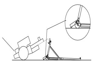
Lock the safety arm in place before operating the machine. **DO NOT** work on any machine supported by the Jungle Jack without the safety arm in position.
