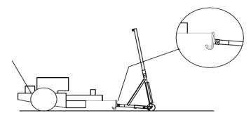
Securely connect the Jungle Jack to the mower deck with the hook as shown.
