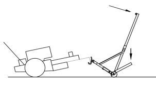
Apply steady force to the handle to initiate lifting. For heavy machines use the foot assist pedal to aid lifting.
