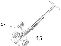
When the Jungle *Jack is in the raised* position, remove the clevis pin (17) and hitch pin (15) from the assembly.
