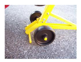
Refer to the following illustrations for the proper placement of the Jack Tooth under the mower deck or rear frame. This will ensure proper weight distribution to avoid possible tipping.
