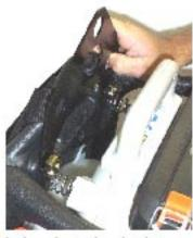
Slide the adaptor brack et between the bracket on the spring and the plastic back of the blower.
