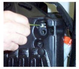
Secure the adaptor bracket using the 10-32 x 1" socket head cap screws, split ring lock washers, and finally, the flat washers provided with your adaptor bracket. You will also need to re-install the oval spacers between the bolt and the plastic backing.
