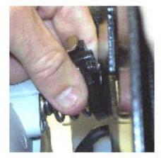
Be sure the extrusions on the spring bracket fit into the holes of the adaptor bracket.
