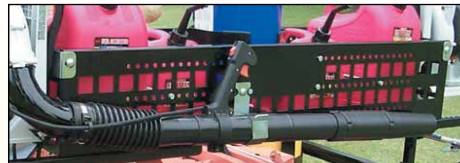
Support brace for blower tubes
