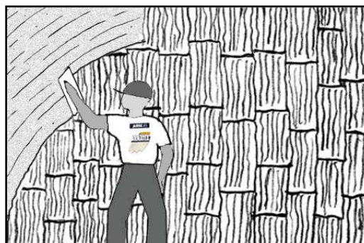
(diagram.3) smooth off and remove excess
