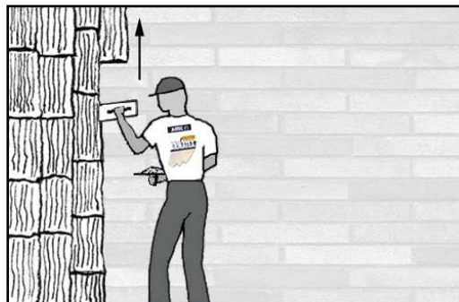
(diagram.2) transfer the Pre-patch to the wall
