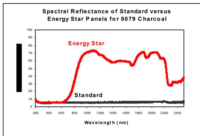
Energy Star coatings have increased durability and life expectancy compared with conventional paints. Independent laboratory testing to ASTM Standards confirmed Solar Reflectance Indices of 241% greater than normal paints on a dark colour like Slate Grey.
