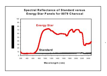
Energy Star coatings have increased durability and life expectancy compared with conventional paints. Independent laboratory testing to ASTM Standards confirmed Solar Reflectance Indices of 241% greater than normal paints on a dark colour like Slate Grey.
