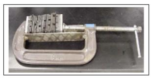
Hot-Tyres-Pickup Test is done in 120F oven over period of 90 minutes. 2x2 inch squares of tyres and paint coated substrate are pressed together by way of 6-inch industrial clamp - as on the attached picture. Compression pressure = 5 x 360 deg twists of screw. The substrate that we use is: Black Leneta Wet Adhesion/Scrub Test Panels.
