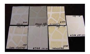
Hot-Tyres-Pickup Test is done in 50 C oven over period of 90 minutes. 2x2 inch squares of tyres and paint coated substrate are pressed together by way of a 150 mm industrial clamp - as on the attached picture. Compression pressure =  $5 \times 360$  deg twists of screw. The substrate that we use is: Black Leneta Wet Adhesion/Scrub Test Panels.
