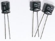
22u cap. (1) 47u cap. (2) [1 goes in top right 10u slot] 10u cap. (1)
