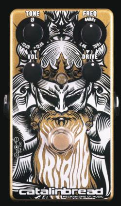
FREQ: This control is part of the original VariOboost circuit, and Freq and Tone work in tandem. Freq selects a frequency between 70Hz and 1.4KHz, which is then cut or boosted by the Tone control. See diagram on the next page if this makes no sense right now.
