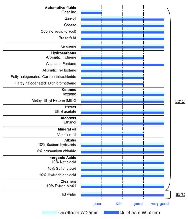
Poor = Will result in severe degradation - Not recommended
