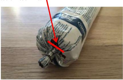
**<u>DO NOT</u>** cut the entire crimped end off the sausage as this will allow Glue to penetrate into the sausage gun cylinder causing a glue blockage and potentially a stuck sausage in the cylinder that is difficult to remove.
