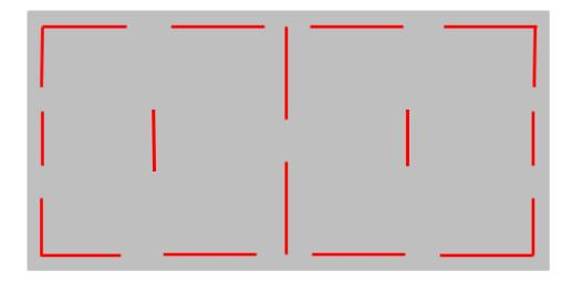
For heavier panels at over 2kgs per m2 such as Quietspace Panels and Cube more glue is recommended and should be applied as below. Applying a 7mm glue bead as shown below will use approximately 5 linear metres of glue on a 1200 x 600mm size panel.
