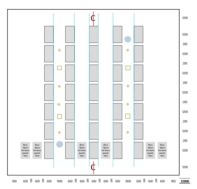
Mark the centre points across the room in the same way by measuring the length of the room and find the centre point; which should be at 6 metres if the room is excactly 12 metres wide.
