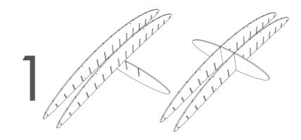
Sort the Lattice 'fins' into pairs, then into size order: largest to smallest. Start by taking one of the largest fins and slotting it into place in the 'rail'.
