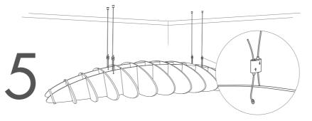
Lift the Lattice up to meet the cables and loop the wires through the plugs followed by the "Velda" cable clips.
