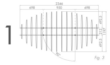
Determine where you want the Lattice to hang (Fig. 3). Mark the ceiling mount points as per the dotted lines.
