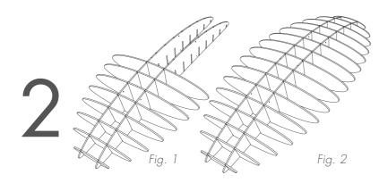
Finish one side by methodically inserting one of each pair into place in order of decreasing size (Fig. 1). Repeat for the other side (Fig. 2).
