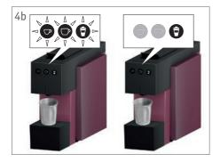
**5** Press the rinse/milk button to activate the rinsing process. The rinse/milk button will blink during the rinsing process, and all the button symbols will illuminate when it is complete.
