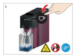
NOTE Exact water quantities dispensed in steps 4 and 5 will depend on the machines current programmed cup capacity. To meet minimum volumes in step 4 and 5 reset factory settings (page 15) prior to cleaning process.
