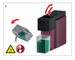
7 Now press the "Large cup" button again to rinse the appliance out with fresh water (do not insert a capsule!). Repeat this process until the water dispensing from the spout is clear.
