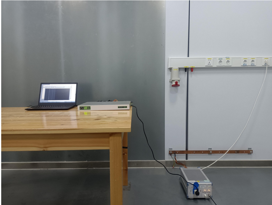
Radiated Emission Test Setup
