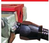
Push the olive on the hose against the side of your vice or a strong flat surface. Look inside the PTFE liner and ensure it is seated and square inside the olive.
