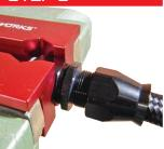
Push the hose over the nipple on the hose end, and engage the threads. Be careful not to cross thread
