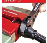
Using an AN spanner, tighten the hose / socket on the hose end, until there is a gap of approximately 1mm between the socket and hose end.
