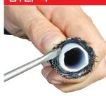
Use a flat screwdriver to carefully separate the braid from the PTFE liner, ensuring you don't damage the PTFE liner in the process.
