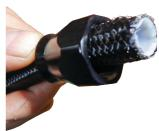
Undo the socket from the hose end and slide socket over the hose, taking note of which end of the socket is threaded and needs to be joined to the hose end.
