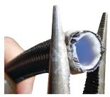
Ensure the hose is round by gently squeezing with pliers. Remove tape from hose.
