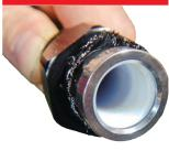
Slide the olive, tapered-end-first over the PTFE liner, under the braid. Make sure there is no braid between the PTFE liner and the olive.
