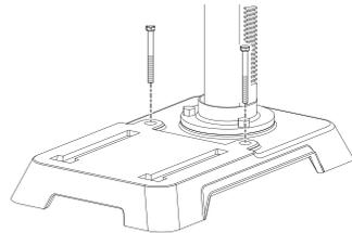
**NOTE:** All bolts should be inserted from the top. Install the lock washers and hex nuts from the underside of the workbench.
