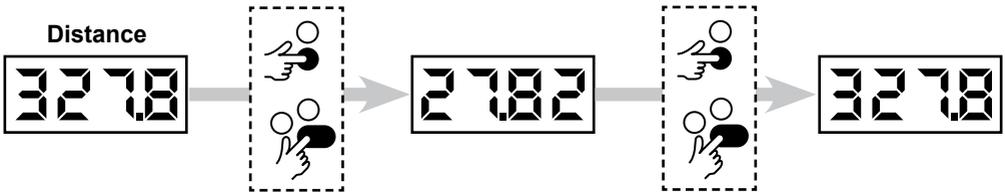
Hold BOTH bottom buttons at the same time until the decimal stops flashing.
