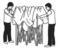
Engage the auto slider at each corner by pushing up with one hand while holding down top of leg with the other hand. Snap Button will engage in
