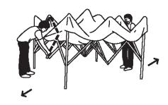
Lift two adjacent outer legs up and pull out the inner legs until snap locks. Repeat on all legs. Raise or level the shelter using adjustment holes found near bottom of each outer leg.
