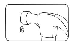
Insert plastic anchors into drilled holes. Lightly tap with hammer until flush with wall.
