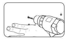
Using a drill and 1/4" (6.35 mm) drill bit, drill two vertical holes for each.
