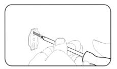
Position the mounting brackets against anchor holes and thread screws until secure.
