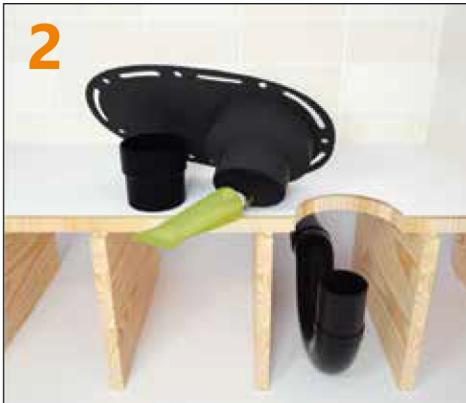
Measure and cut a ABS or PVC piece as needed to ensure a secure connection with the P-trap below. Note that the drain body has an outlet of 2 in. (a coupling reducer of 1 1/2 in. is included).
