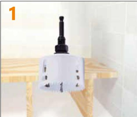
Drill a 4 in. hole into the wood floor.
