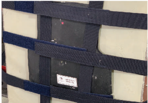
NIJ 0101.06 STANDARD TESTING: 6 SHOTS CLAY ROME #1
