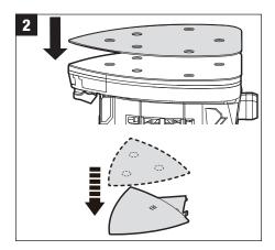
the holes in the sanding base and press firmly into place.d) To remove the sanding paper, peel it away from the base.
