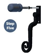
Fit the upper screw into handle and locate thread in the lock with the screw in your fingers before using the screwdriver to tighten.
