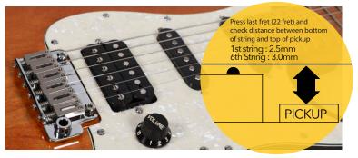
We recommend you try to adjust the height of the pickup using several different ways. This is where your personal taste comes into play. However, if the pickup is too close to the string, the magnet of the pickup may interfere with the normal ringing of the string. Also, if the pickup is too far from the string, the output can be very low. Please adjust it based on the general settings above.
