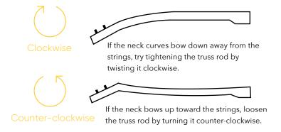
Depending on the guitar, the position of the truss rod may be between the head and the neck, or between the neck and the body. When turning the truss rod, think of it like using a screwdriver.
