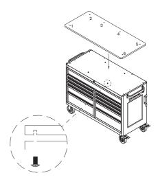
Place the worktop on the floor. Drill six 7/16" (1.1 cm) holes at the locations you marked.
