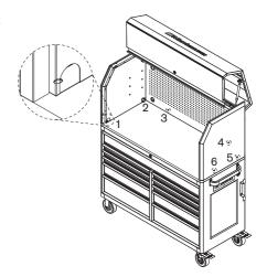
Take the hutch off the cabinet. Remove the worktop by first removing the drawers, then loosening the M6 x 12 Phillips head bolts.
