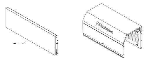
Attach the left and right side panels to the back of the hutch body using three  $M8 \times 20$  hex bolts and washers per panel.
