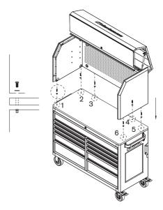
Install the shelf in the hutch using four M8 x 20 hex bolts and washers.
