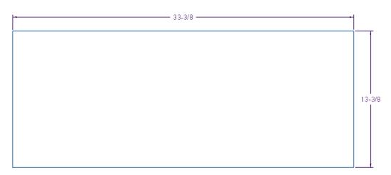
Ensure the wall opening is 33-3/8" x 13-3/8" for proper window fit. Install the window frame into the opening and attached using the 14 screws included.
