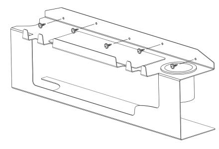
Fasten the shelf to the wall section using the 5 supplied sheet metal screws. Recommended height is 4-1/2" below the window. \*\*Do not overtighten\*\*
