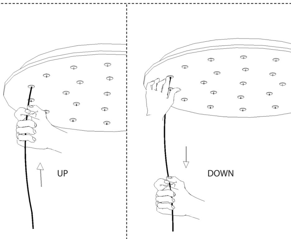
**6** To adjust wire lengths: **NEVER TUG ON WIRES!** The fixture comes assembled at the maximum length. Lengthening a wire can only be done once it has been shortened. Never try to lengthen wires past the maximum length.
