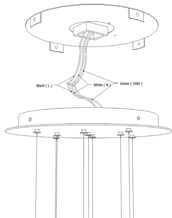
**3** Make the electrical connections to the corresponding wires, then re-attach ceiling mounted bracket to the canopy using provided screws.
