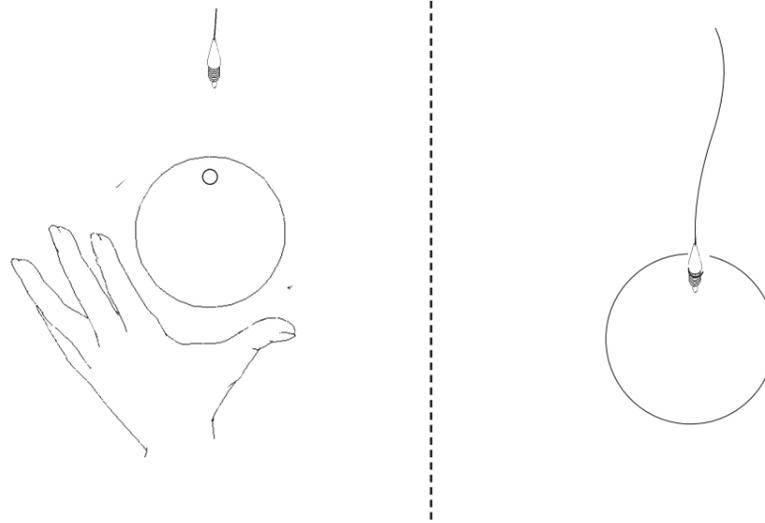
**7** Once the fixture is mounted and wires have been adjusted, attach your glass pendants. Ensure sockets are cool to the touch before proceeding.
