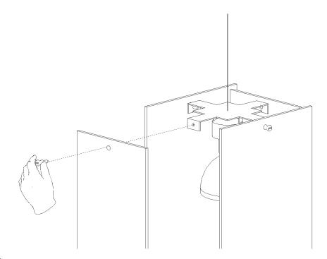
Once the fixture is hanging and wires have been adjusted, attach your glass pendants. Ensure sockets are cool to the touch before proceeding.
