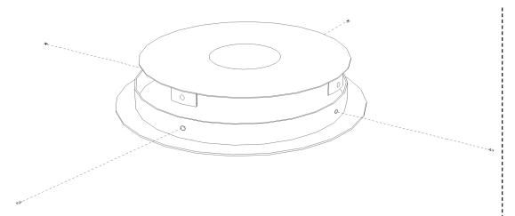
Ensure there is no power feeding to the fixture before starting. Remove provided screws from canopy/bracket, then remove the bracket from the canopy.
