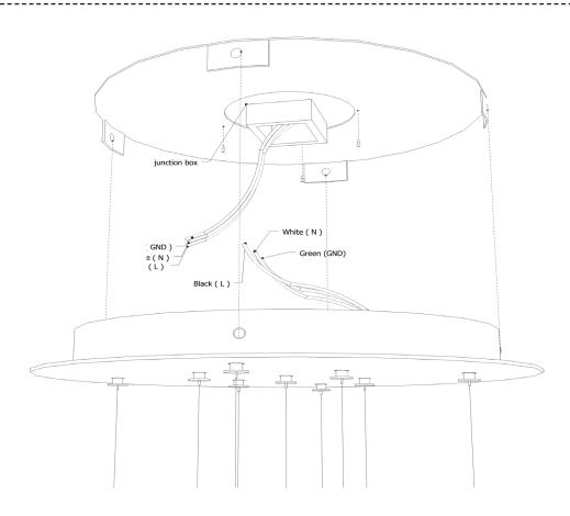
2 Install the metal bracket to the ceiling using (customer provided) screws, anchors and fasteners.
