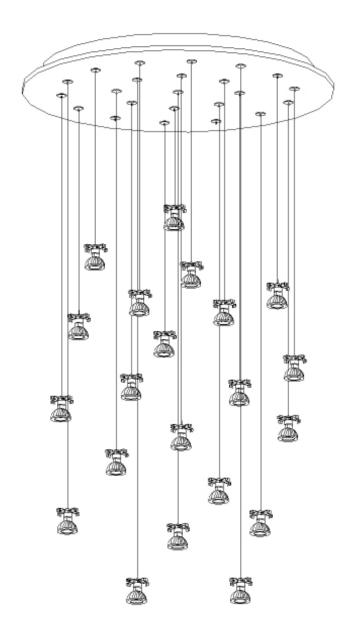
7 You are able to make adjustments to the wire lengths if necessary using the provided metal grippers on the canopy. SEE BELOW.
