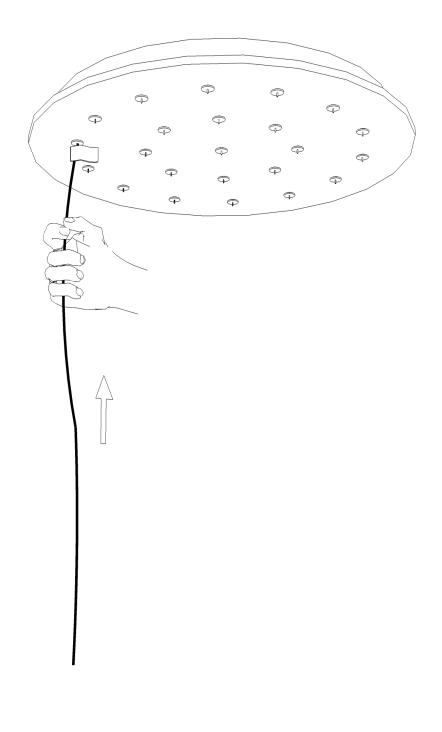
**6** Push each wire up untill the flag reaches the canopy , and remove the flag. This will match the pre determined drawings (Inclosed).
