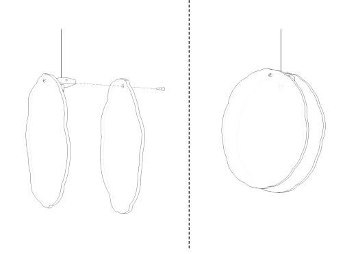
8 Once the fixture is hanging and wires have been adjusted, attach your glass pendants. Ensure sockets are cool to the touch before proceeding.
