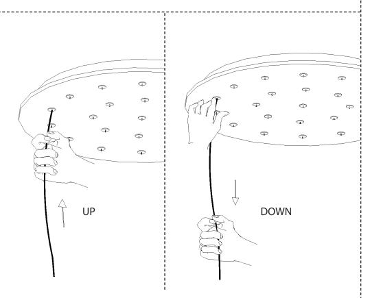
To adjust wire lengths: NEVER TUG ON WIRES! The fixture comes assembled at the maximum length. Lengthening a wire can only be done once it has been shortened. Never try to lengthen wires past the maximum length.
