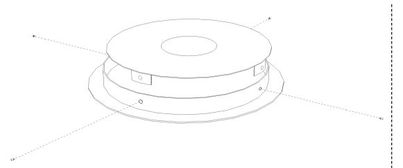
1 Ensure there is no power feeding to the fixture before starting. Remove provided screws from canopy/bracket, then remove the bracket from the canopy.
