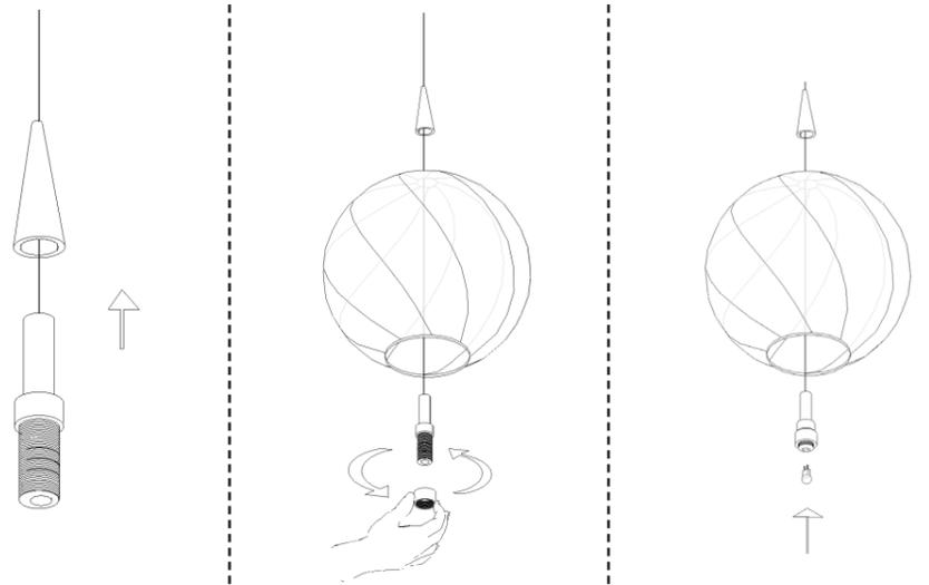
**8** Once the fixture is hanging and wires have been adjusted, attach your glass pendants. Ensure sockets are cool to the touch before proceeding.
