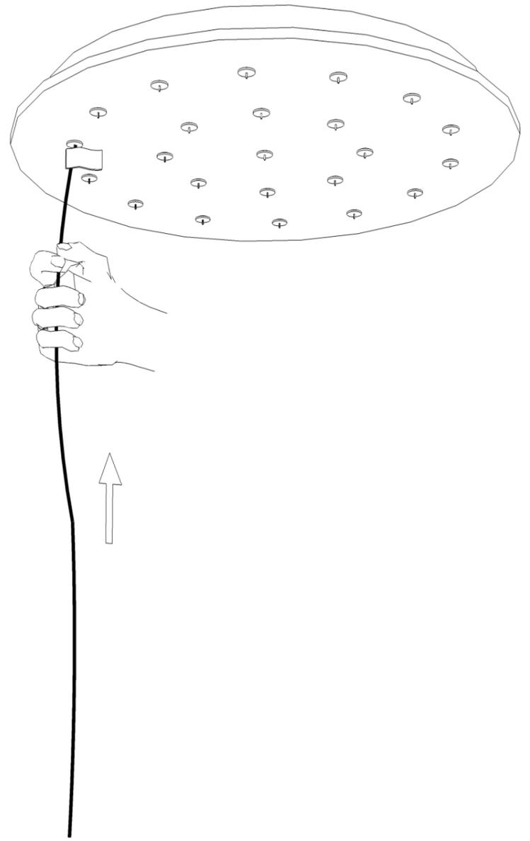
**6** Push each wire up until the flag reaches the canopy , and remove the flag. This will match the pre determined drawings (Inclosed).
