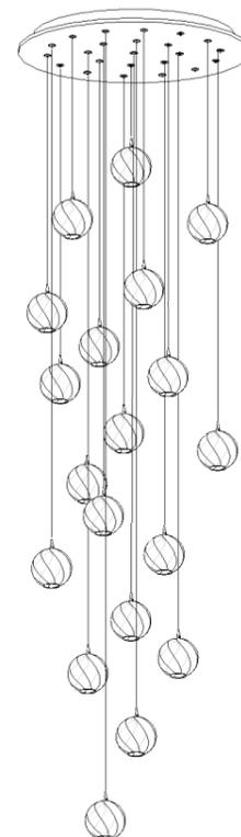
**10** Once all pendants are hanging, carefully make any final adjustments to the wire lengths as necessary to get the desired look.
