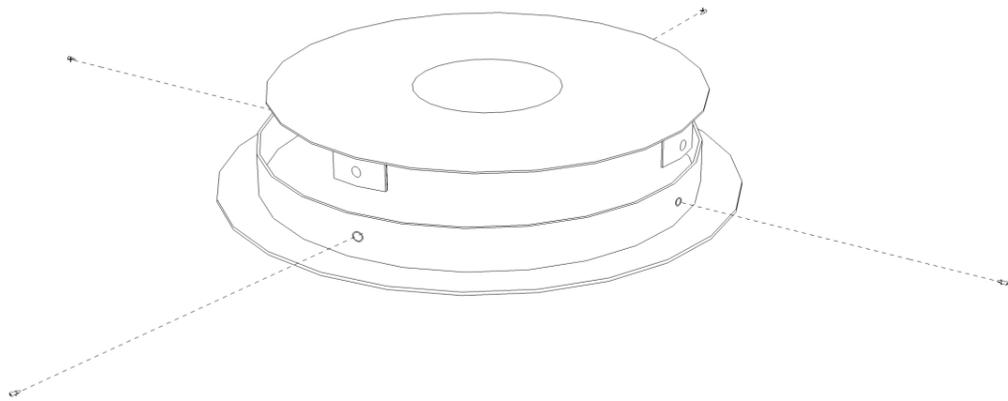
**1** Ensure there is no power feeding to the fixture before starting. Remove provided screws from canopy/bracket, then remove the bracket from the canopy.
