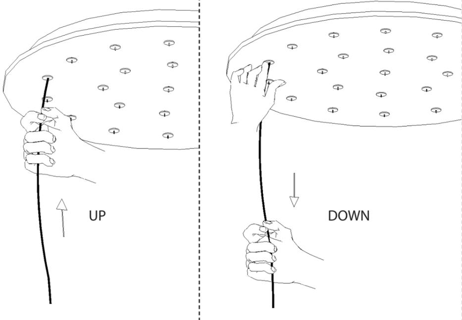
To adjust wire lengths: NEVER TUG ON WIRES! The fixture comes assembled at the maximum length. Lengthening a wire can only be done once it has been shortened. Never try to lengthen wires past the maximum length.
