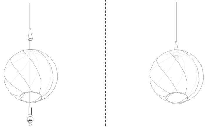
**9** Once socket, nut and bulb are assembled, gently lower the glass pendant pulling the wire through until the upper tip of the socket goes through the top hole, then lower the metal cone to cover the socket tip.
