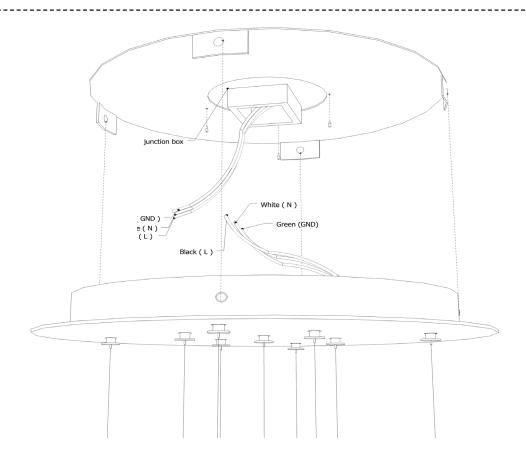
2 Install the metal bracket to the ceiling using (customer provided) screws, anchors and fasteners.
