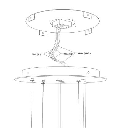
3 Make the electrical connections to the corresponding wires, then re-attach ceiling mounted bracket to the canopy using provided screws.
