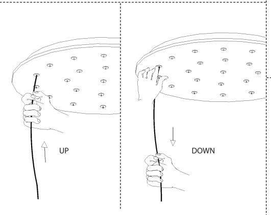
To adjust wire lengths: NEVER TUG ON WIRES! The fixture comes assembled at the maximum length. Lengthening a wire can only be done once it has been shortened. Never try to lengthen wires past the maximum length.
