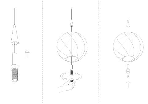
8 Once the fixture is hanging and wires have been adjusted, attach your glass pendants. Ensure sockets are cool to the touch before proceeding.
