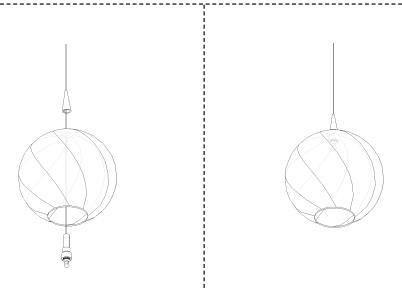
**9** Once socket, nut and bulb are assembled, gently lower the glass pendant pulling the wire through until the upper tip of the socket goes through the top hole, then lower the metal cone to cover the socket tip.
