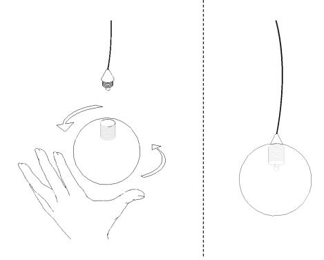
7 Once the fixture is hanging and wires have been adjusted, attach your glass pendants. Ensure sockets are cool to the touch before proceeding.
