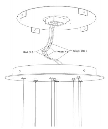
3 Make the electrical connections to the corresponding wires, then re-attach ceiling mounted bracket to the canopy using provided screws.
