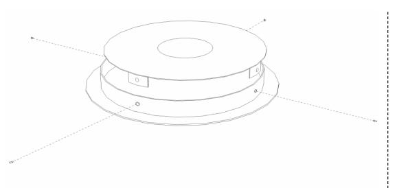
1 Ensure there is no power feeding to the fixture before starting. Remove provided screws from canopy/bracket, then remove the bracket from the canopy.
