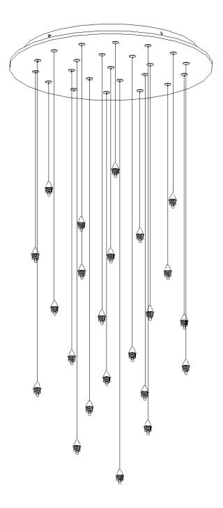
**5** If your chandelier is not pre-staggered (most standard length fixtures are not), stagger it to the desired design. You are able to make adjustments to the wire lengths if necessary using the provided metal grippers on the canopy. SEE BELOW.
