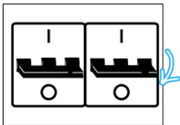
Turn off the power at the circuit breaker for the outlet you are replacing.
