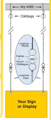
Keeping the Pole vertical, extend it to the FlatHat height. Attach one ClikMagnet to the metal in a FlatHat, then walk to the next FlatHat location and repeat. Clik-Clik—Your Sign is Hung!
