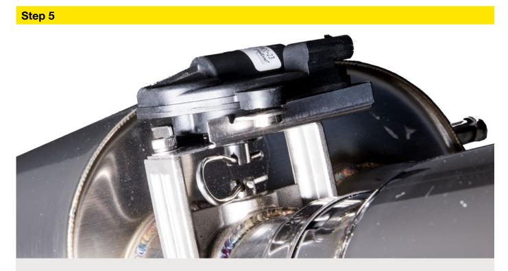
Remove your OE valve-motor from the OE exhaust by undoing the three locating bolts. Push it into place on your new exhaust valve. The two slots should now be aligned, as shown.
