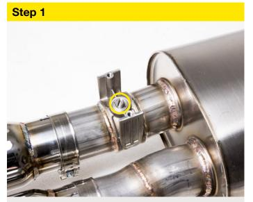
Using a flat-blade screwdriver, turn the valve so it is in the open position.
