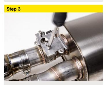
Place the exhaust valve plate in place (as shown) and secure to the valve-motor assembly with the two supplied bolts.
