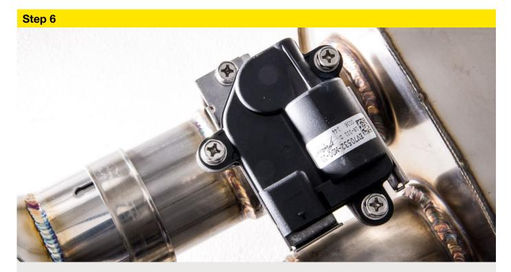
Once the link rod is seated correctly on both sides (this will be an interference fit), tighten the three valve-motor locating bolts - you're ready to install your new mountune exhaust.
