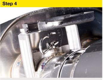
With the valve in the open position, push the link rod into place on the valve cut-out, as shown.
