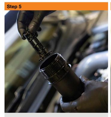
Remove the plastic filter locating tube from the OE housing by firmly, but carefully pulling it out.
