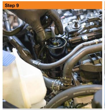
Carefully screw the housing in to place making sure it is not cross threaded.
