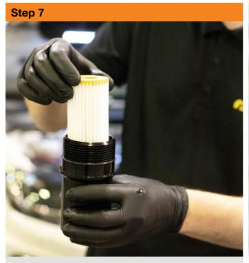
Although the original filter can be reused at this point, it is recommended that a new filter is fitted. Slide the filter on to the locating tube and push firmly in to place. <image>
