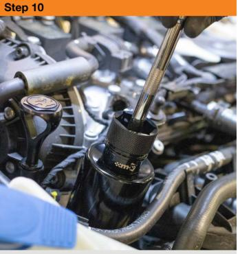
Using a torque wrench and the supplied m52 socket, tighten the housing to 25nm (18ft/lb).
