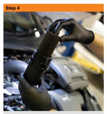
Remove the oil filter from the OE housing, and if replacing with a new filter, dispose of the old one in accordance with your local regulations.
