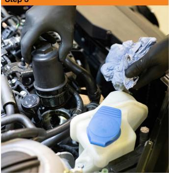
Remove the filter housing from the engine. Cover the bottom of the oil filter housing with some rag or tissue before moving across the engine bay to catch any spills.
