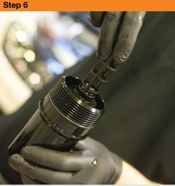
Fit the filter locating tube in to the m52 oil filter housing, making sure it clicks in to place.
