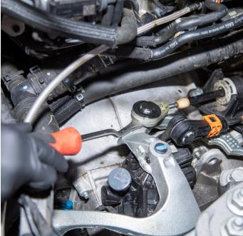
Making sure the vehicle is in 4th gear, use a trim tool to remove the gear cable.
