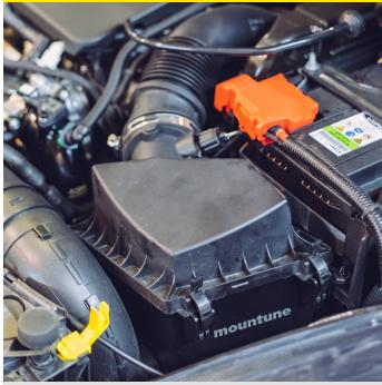
Once installed proceed to refit the airbox/ intake by reversing the previous steps used to remove.
