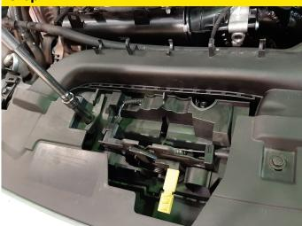
Remove two 10mm screws from the front panel.
