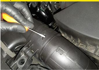
Depress the locking tab from the air intake. There are two tabs, one located on the top of the intake and one underneath.
