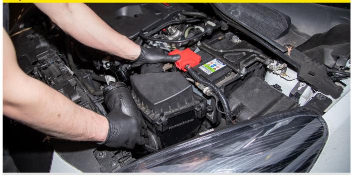
Remove the air box by pulling it upwards, please ensure that the air box base grommets remain in place.
