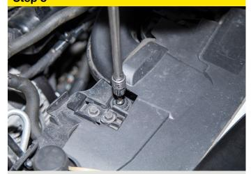
Remove two Torx 30 screws from the air intake.
