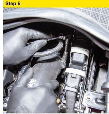
Using the a hose clip driver or flatbladed screwdriver loosen the hose clip enough for the induction hose to be removed.
