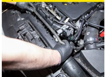
Unclip coolant hose from air intake.
