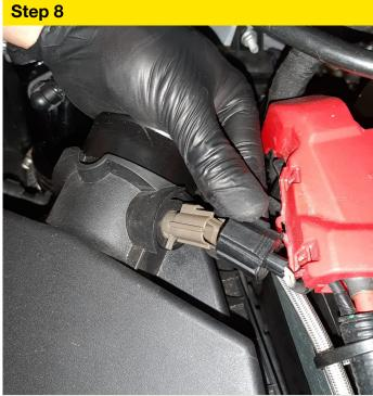
Remove the MAF sensor plug.
