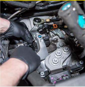
The rollpin can now be removed using an appropriate hammer (a 12oz hammer is recommended) and the supplied drift. Strike the roll pin with the drift until it is fully removed.
