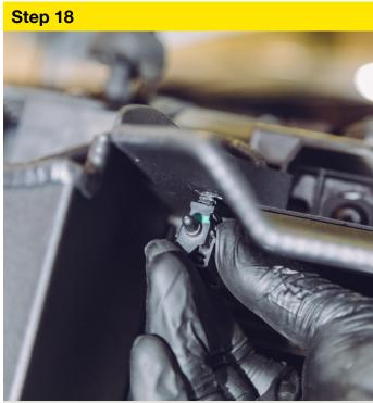
Refit the ambient air temperature sensor from the underside of the shroud as shown.
