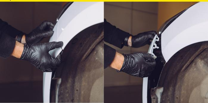
Carefully pull the side of the bumper as shown away the from the wheel arch until it is clear of the vehicle. Do this for both sides of the bumper.
