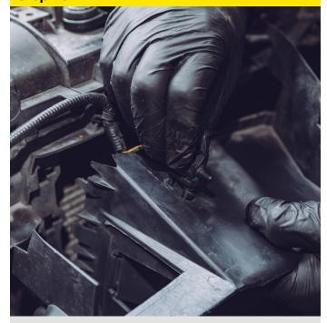
Gently remove the ambient air temperature sensor.
