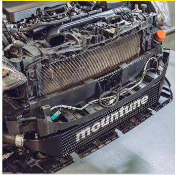
Remove the original shroud from the front of the vehicle.
