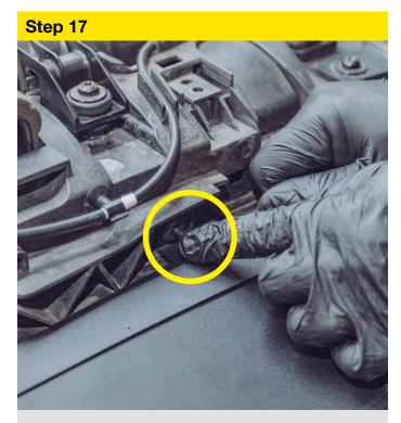
Push in the original fasteners on either side of the ACAI as shown.
