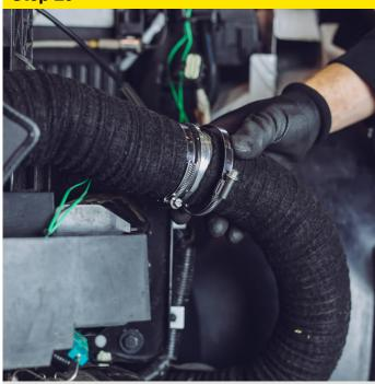
If you are running the mountune Induction Kit attach the ACAI supplied shannon hose to the air box shannon hose using the supplied coupler and jubilee clips as shown.
