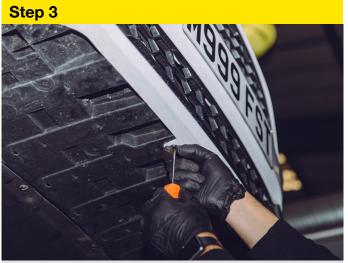
Next, using a phillips head screwdriver undo the 6 plastic fasteners that connect the bumper to the undertray.
