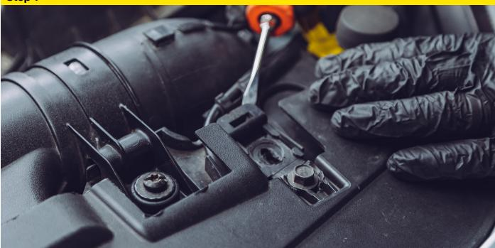
Lift the tab on the top of the slam panel up on both sides.
