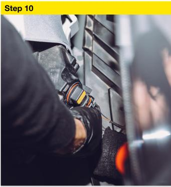
Gently remove the fog light connectors on both sides, then remove the bumper from the vehicle.
