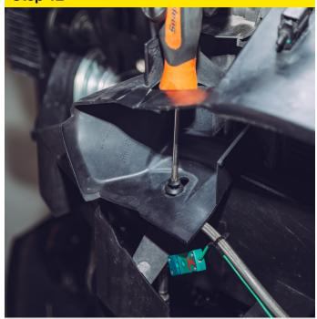
Now using the same screwdriver remove the lower self tapping screws from both sides of the shroud.
