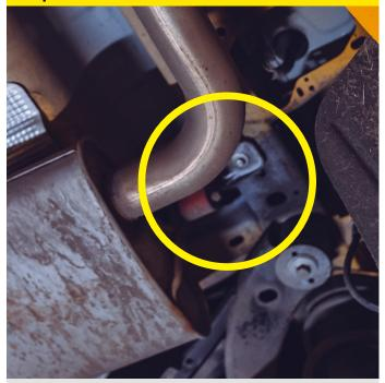
You will then need to remove the original OE exhaust silencer by removing the 2x 10mm bolts securing the exhuast to the chassis.
