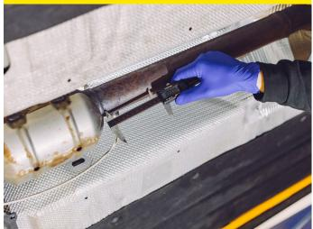
Measure 100mm from the bottom weld of the GPF and mark this with a pen.
