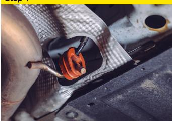
Remove the exhaust hangar bush located on the first bend.
