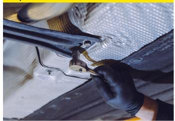
Use a 13mm socket and ratchet to remove the exhaust brace from the underside of the vehicle.
