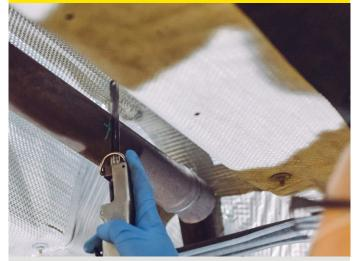
Using an airsaw/hacksaw cut through the exhaust pipe on your mark.
