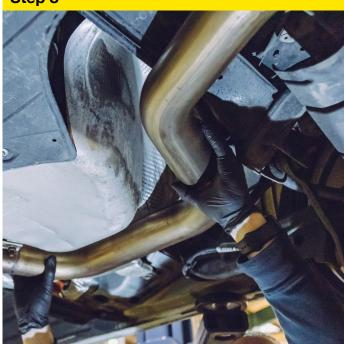
Now you can take the exaust section with the two bolt flange and place into position, connecting it to the silencer as shown.
