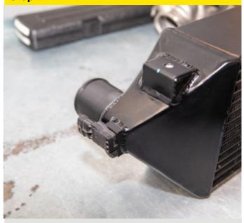
Using the supplied set screw, fit the MAP Sensor in to the mountune intercooler. Care must be taken to not overtighten the screw.
