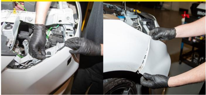
Unclip the two bumper securing tabs in the headlight apertures. Carefully but firmly pull the end of the bumper out and away from the wing. It only needs to move approx. one inch, pulling any further than this may cause damage.
