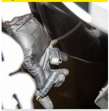
Once you have removed the bumper approximately 4-5 inches, reach down behind the left hand headlight and disconnect the front fog light wiring harness multi plug.
