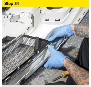
Replace the standard clips to secure the plate. A pair of long-nose pliers can help with this.
