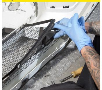
Slide the mountune blanking plates into place. The foam should face the intercooler.
