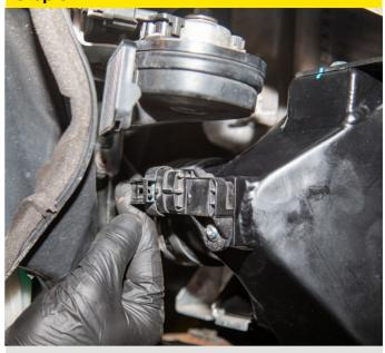
Reconnect the MAP sensor wiring harness multi plug.
