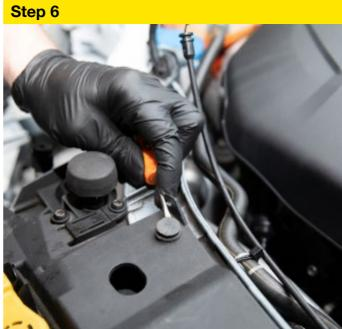
Using a trim tool, remove the two push clips from the top of bumper.
