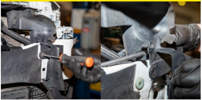
Undo the two T30 screws securing the intercooler ducting and remove.
