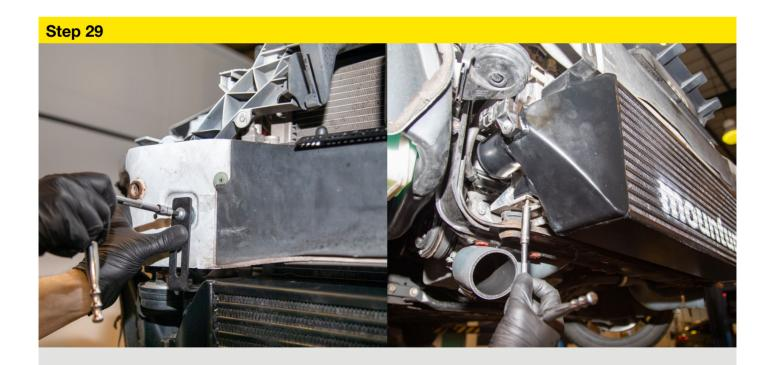
Tighten the two bolts on the new top fasteners, followed by the two 8mm headed bolts in the bottom.
