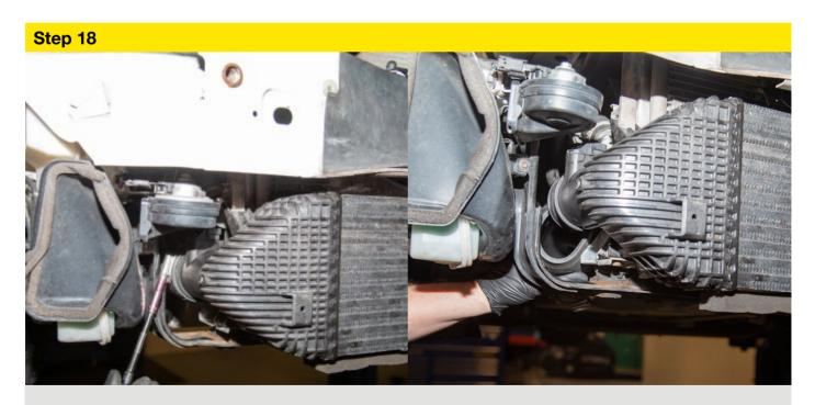
Loosen both hose clips and remove the intercooler hoses. Carefully tuck them out of the way. Note: It is good practice to cover the ends of the hoses with a cap or tape to prevent dirt/grit entering the engine.
