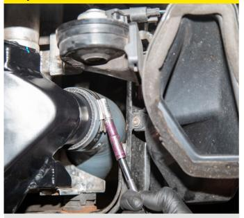
Reconnect both boost hoses and secure with the supplied hose clips.
