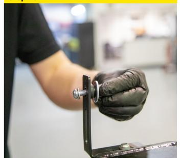
Loosely fit the supplied fastener to the L-bracket using the supplied bolts and washers. Fit a washer to the back side of the fastener as shown.
