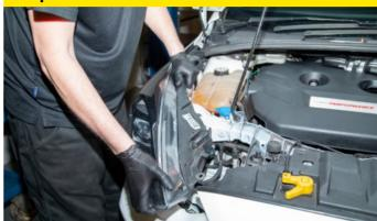
Twist and pull up on each headlight to remove, and disconnect the wiring harness.
