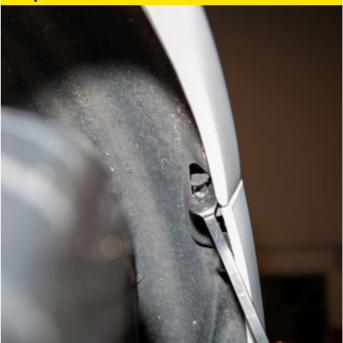
Using a trim tool, remove the two trim clips from inside the wheel arches.
