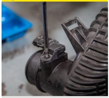
Undo and remove the Torx screw securing the MAP sensor into the intercooler. Carefully remove the sensor by pulling firmly, but gently away from the intercooler.
