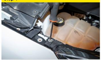
Undo and remove the two T30 Torx bolts from each headlight.
