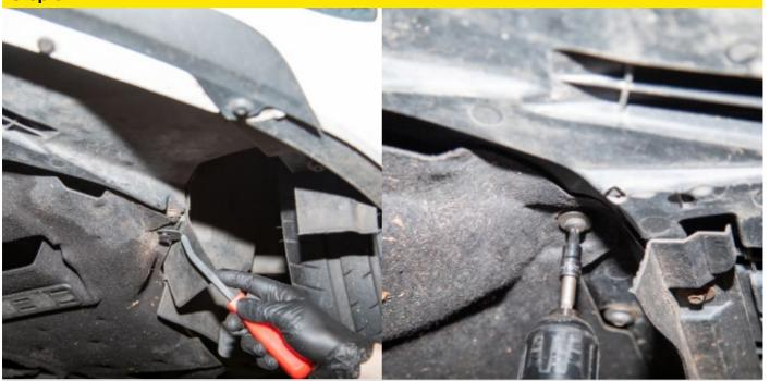
With the vehicle supported on a ramp or axle stands, remove all the T30 Torx screws and the two outer trim clips securing the engine under tray.
