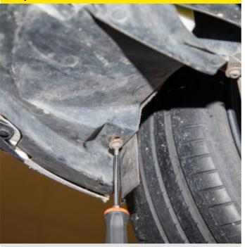
Undo and remove the seven T30 Torx screws from the bumper undertray.
