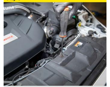
Undo the three T30 Torx screws from the middle of the bumper trim.
