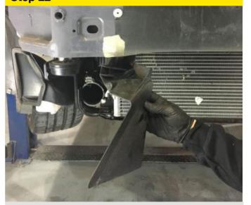
Unclip and remove the standard intercooler ducting from the cooling pack. Note: It may be necessary to loosen the four 10mm headed bolts holding the cooling pack to give more room to remove. If lowering the cooling pack, ensure the assembly is supported with a jack or stand to avoid damage to the hoses or wiring. This ducting will not be refitted.
