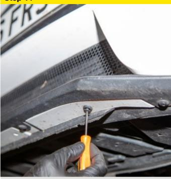
Carefully unscrew and remove the plastic trim clips from the front edge of the bumper.
