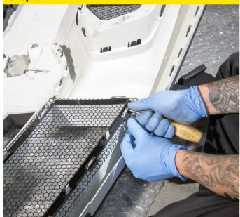
With the bumper on a soft surface, carefully use a screwdriver or trim tool to remove the outer clips from the lower grill.
