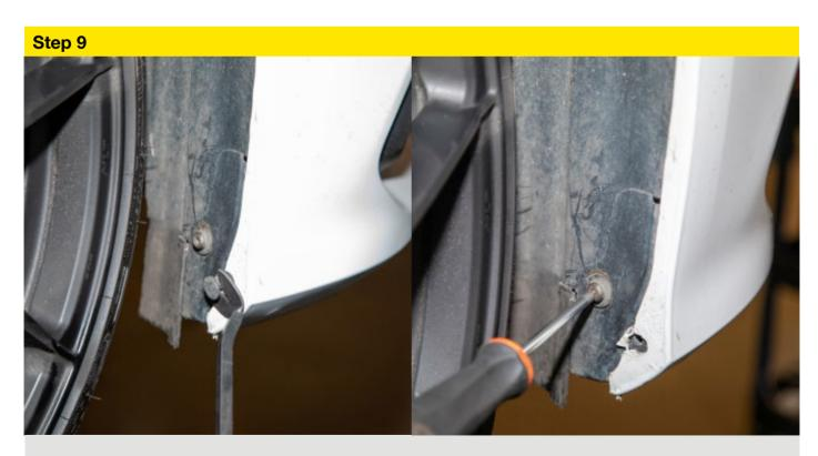
Turn the steering to gain access to the wheel arch liner. Undo and remove the two T30 screws and one trim clip securing the arch liner to the bumper.
