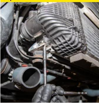
Undo and remove the two 8mm headed bolts from the bottom of the intercooler.
