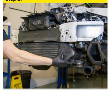
Carefully lift the intercooler assembly approx. half an inch. Pull the lower half of the intercooler away from the radiator and lower to remove from the car.
