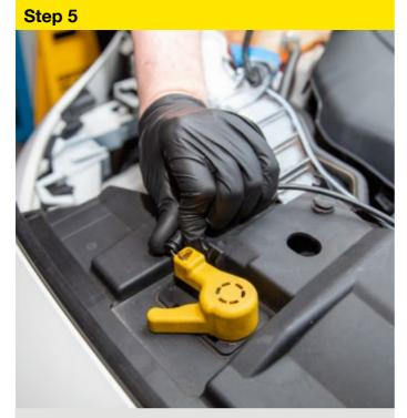
Unclip and remove bonnet cable, DO NOT close bonnet with the cable disconnected.
