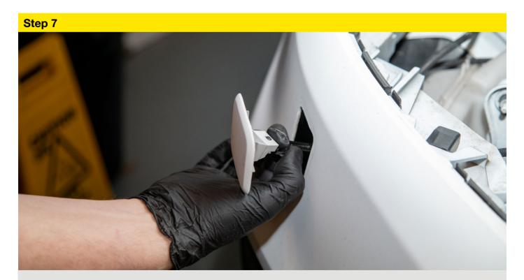
Pull out the headlight washers and remove the cover. This is done by tilting the cover upwards to unclip it from the washer jet. The jet will then retract back behind the bumper.
