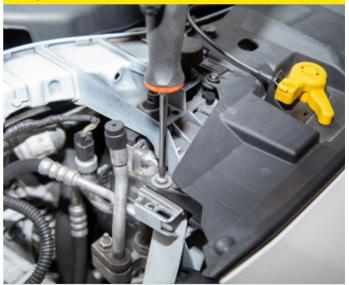
Remove two outer T30 screws from the top of the bumper.
