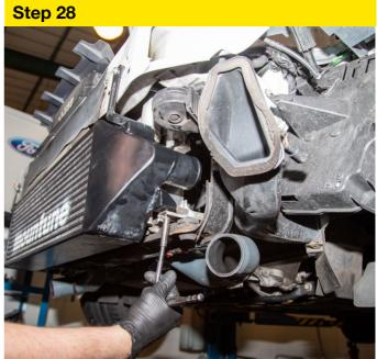
The bottom mounts will line up with the standard mounting point on the radiator. Loosely secure the intercooler using the original bolts.
