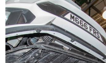
Carefully remove the under tray. It may be necessary to gently flex the tray to disconnect it from behind the bumper.
