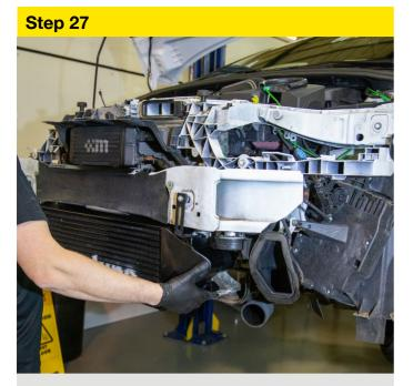
Fit the intercooler in place on the car, position the new fasteners in to the holes on the cross-car beam.
