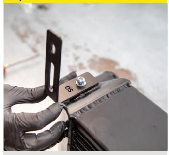
Fit the supplied L-bracket to the intercooler as shown. Secure with the supplied bolts and washers.
