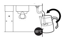
Insert the wand all the way down and tilt
